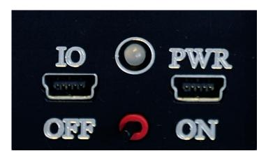
Fig. 2 Interface (IO) and power (PWR) connectors of the labZY Devices.
